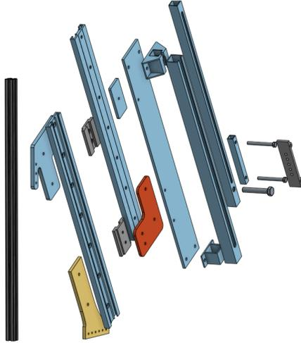
*Picture: Slider design (square extrusions, linear guides, and adapters)*
